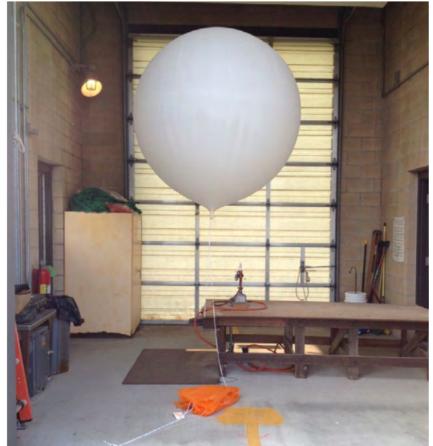
A weather balloon is shown completely inflated, along with its parachute and the instrument package, known as a radiosonde.
